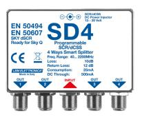
In cases where two or more decoders share the same SCR/dCSS output, Smart Splitters fulfil two important functions: they avoid 'collision' of the commands sent by storing them and then sending them in the correct sequence, and they eliminate criticalities due to the different voltages supplied by the decoders.
