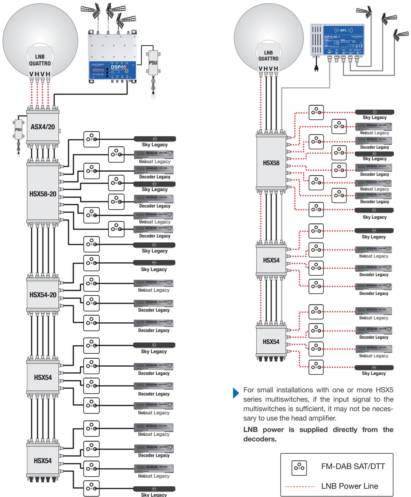
▶ For small installations with one or more HSX5 series multiswitches, if the input signal to the multiswitches is sufficient, it may not be necessary to use the head amplifier.
