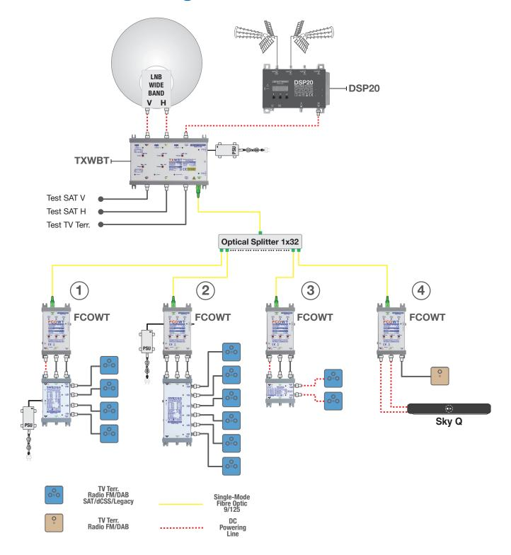
The **TXWBT** headend converts and transmits over a single-mode optical fibre cable the terrestrial signals (DTT, FM, DAB) and all the transponders of a satellite received from an Wide Band LNB. The conversion of the optical signals are performed by **FCOWT**. In the sample there are four suggested use and powering mode of the **FCOWT**:
