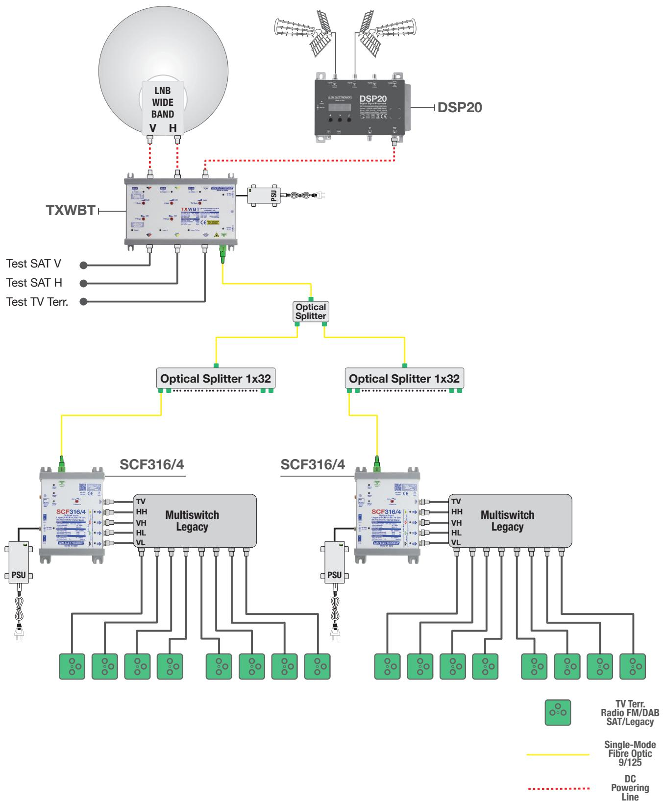
**Distribution of a satellite and terrestrial feed (DTT; FM; DAB) over a single-mode optical fibre to standard five wire multiswitch.**
