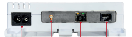
Power Supply 100... 240VAC Earth Terminal Optical Input SC/UPC RJ45 Port
