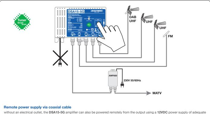
without an electrical outlet, the **DSA15-5G** amplifier can also be powered remotely from the output using a **12VDC** power supply of adequate power such as the **AWF600**.
