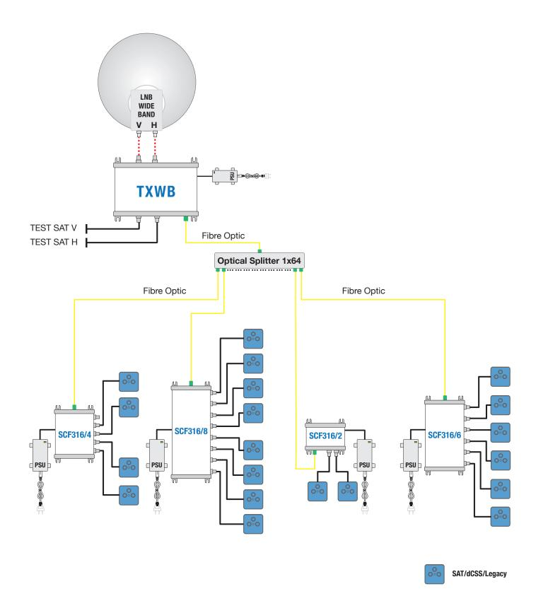
The headend **TXWB** converts and transmits over a single-mode fibre optical cable all the transponders of a satellite received from a Wide Band LNB. The optical signals are received by the **SCF316** series optical multiswitch and converted into RF ready for a single or multi-dwelling coaxial distribution. Each **SCF316** series output provides satellite signals supporting the legacy or SCR/dCSS standards (AUTO-SWITCH).
