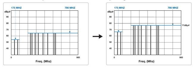
**Example (B):** Scenario with 16 digital TV terrestrial channels plus DAB and FM in a PON (Passive Optical Network) of 32 optical points. The optimal signal level at the **TV Terr. Test** output should be 74dBµV, this level can be set adjusting the **TV Terr. Gain** trimmer.
