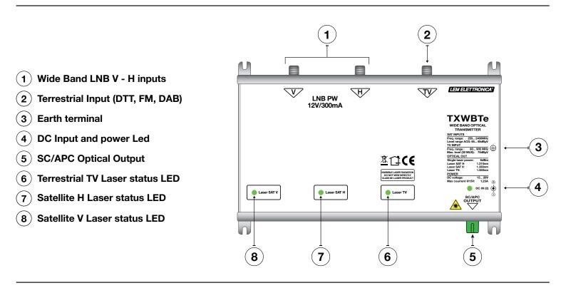
The TXWBTe optical transmitter enables the distribution of satellite and terrestrial TV signals (DVB-T/T2, FM, and DAB) over a single single-mode optical fiber.
